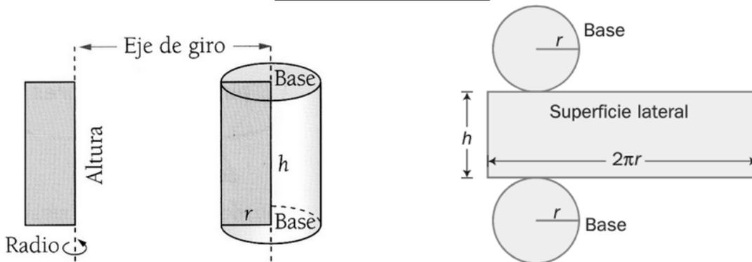
$$A(\text{cilindro}) = 2A(\text{base}) + A(\text{lateral}) = 2\pi r^2 + 2\pi rh \Rightarrow \boxed{A(\text{cilindro}) = 2\pi r(r + h)}$$
