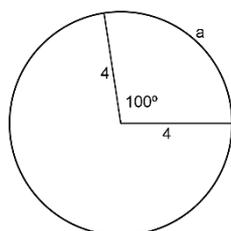
$$\begin{aligned} a &= \frac{2\pi R \cdot \alpha^\circ}{360^\circ} = \frac{2\pi \cdot 4 \cdot 100^\circ}{360^\circ} \cong 6,98 \Rightarrow P(\text{sector}) = 4 + 4 + 6,98 = 14,98 \text{ cm} \\ A(\text{sector}) &= \frac{\pi R^2 \cdot \alpha^\circ}{360^\circ} = \frac{\pi \cdot 4^2 \cdot 100^\circ}{360^\circ} \cong 13,96 \text{ cm}^2 \end{aligned}$$
